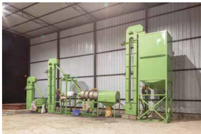
TCTD pilot plant for sand reclamation, commissioned at Govt. Polytechnic, Kolhapur
