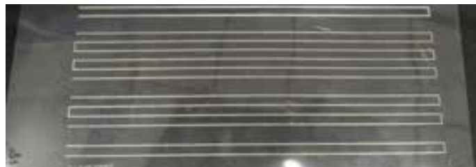
Screen printed conducting silver pattern
