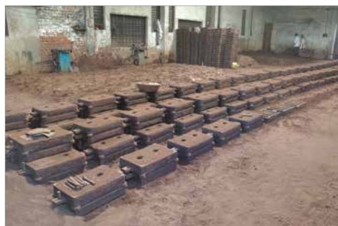
Molds are prepared using reclaimed sand
