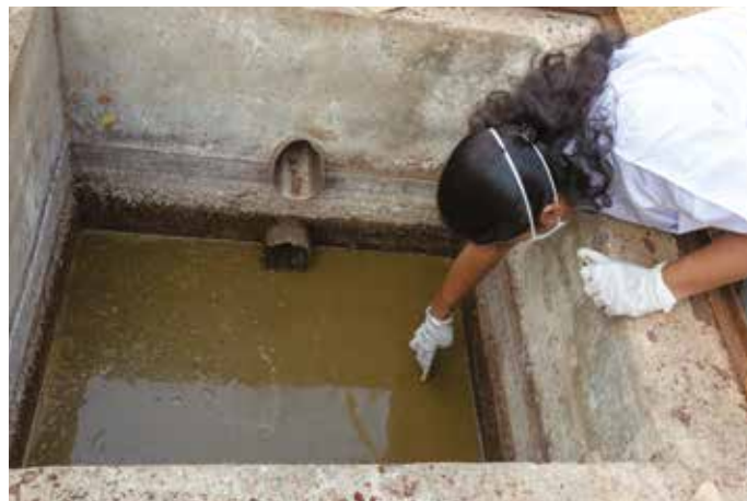
Checking the pH of digested/effluent in outlet tank of anaerobic digester
