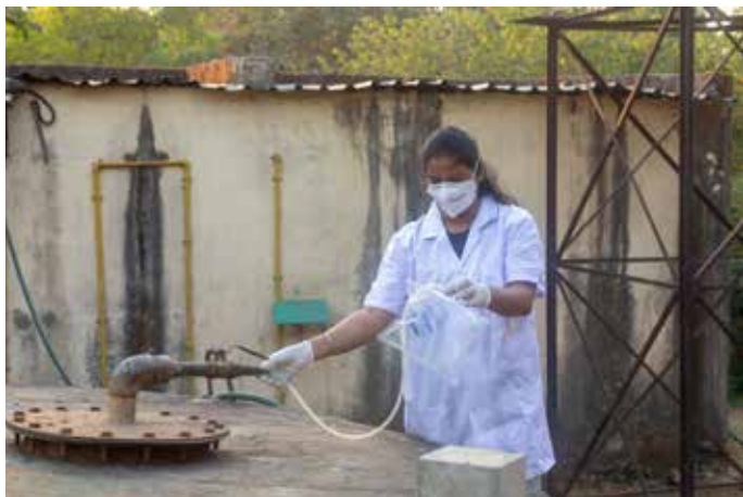
Collection of biogas samples from the biogas plant at IIT Bombay
