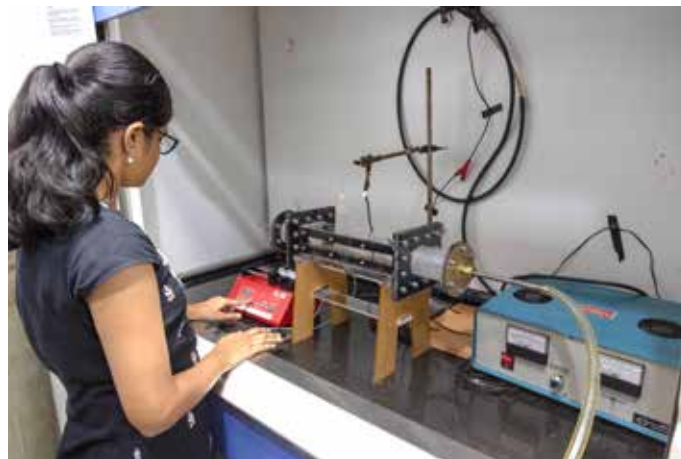
Electrospray based air cleaning system
