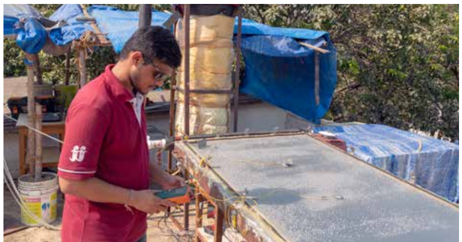
A prototype of the small-scale humidification dehumidification system
