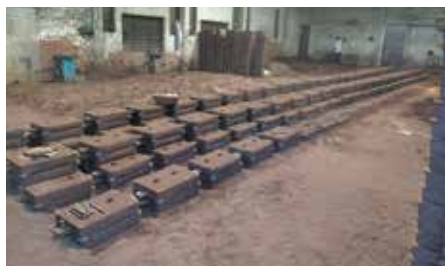
Molds are prepared using reclaimed sand
