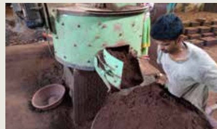
Green sand is prepared using reclaimed sand with the help of sand muller
