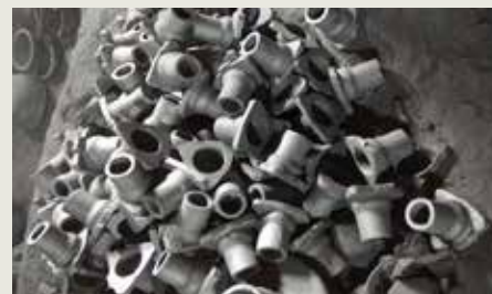
Casting was done using reclaimed sand at Malati Foundry Pvt. Ltd., Kolhapur
