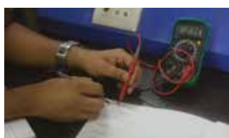
Continuity check of paper circuit
