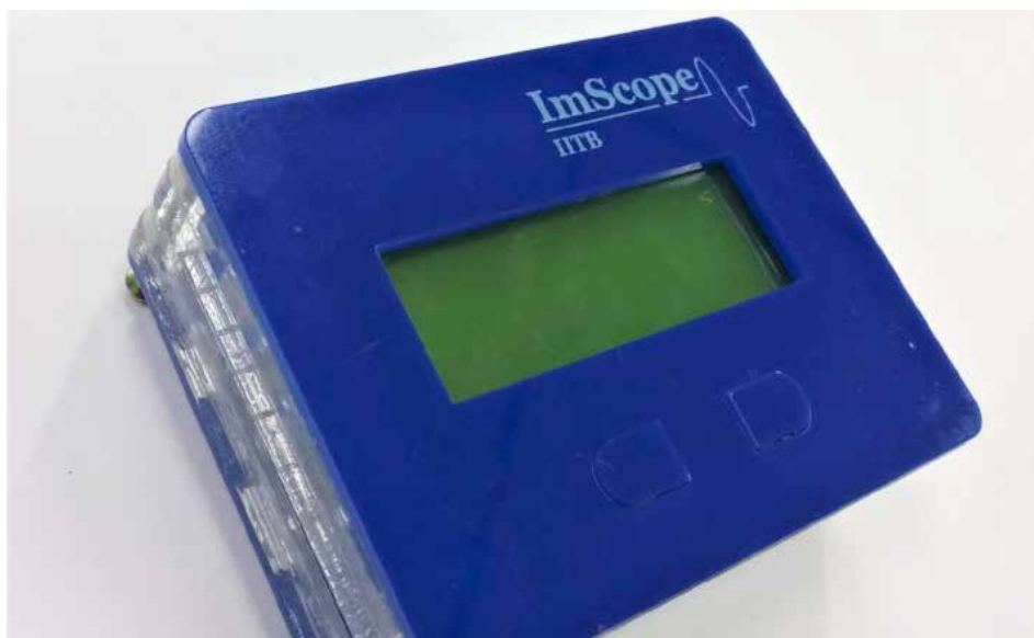
Sensor and electronic system using Electrical Impedance Spectroscopy
