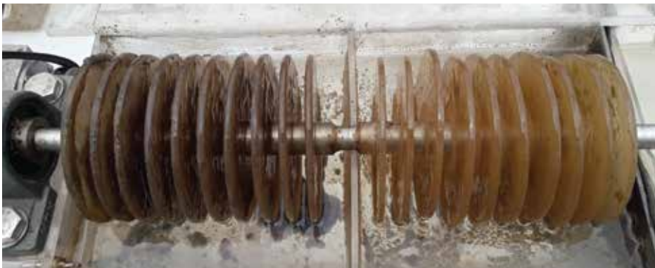
Algae nuisance reduced after covering the reactor
