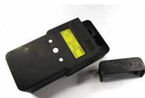
Portable device for heavy metal sensing using optical fibre
