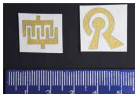
Different configurations of gold electrodes sputtered on filter paper
